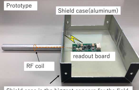
Shield case is the biggest concern for the field shift because of its short distance with coil.
