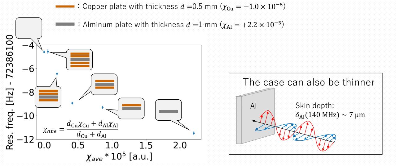
Checked that copper plate, which has -1/2 magnetization as aluminum, can cancel the effect.
