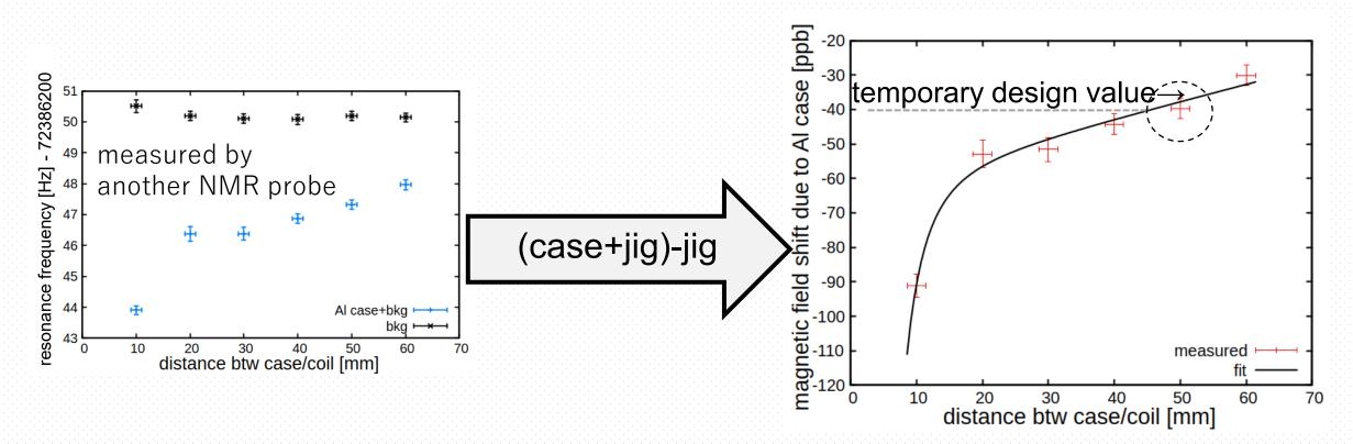
Although systematics with the probe would be calibrated, the less shift value, the better.
