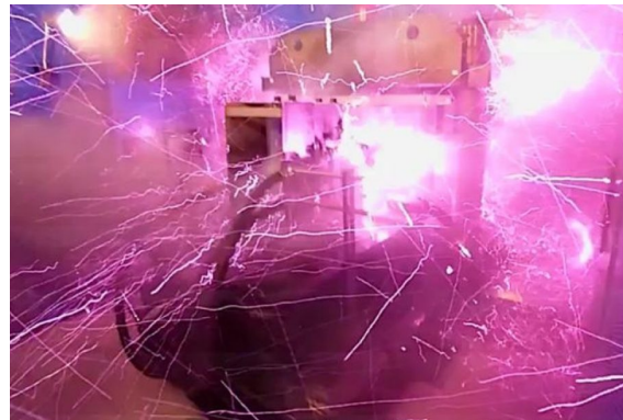
Pulsed Magnet 1200 T, 0.1 ms
