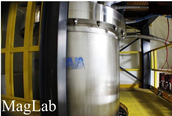
Pulsed Magnet 100 T, 15 ms
