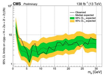
Expected and observed 95% CL limits on  $\sigma(pp \to H) \times B(H \to Za \to 2l2\gamma)$ . The observed (expected) limits range from 17.8 (17.9) fb for  $m_a = 1$  GeV to 4.7 (6.9) fb for  $m_a = 30$  GeV.
