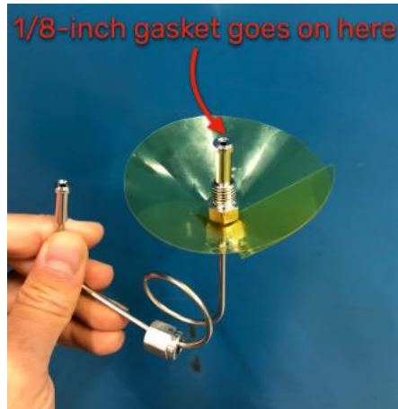
Gasket falling protector made by plastic paper
