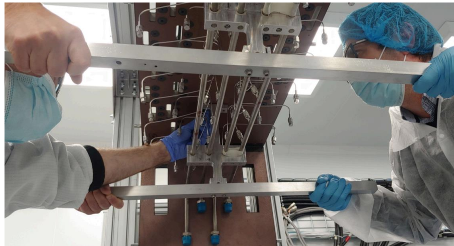
The CO2 cooling pipes are installing
