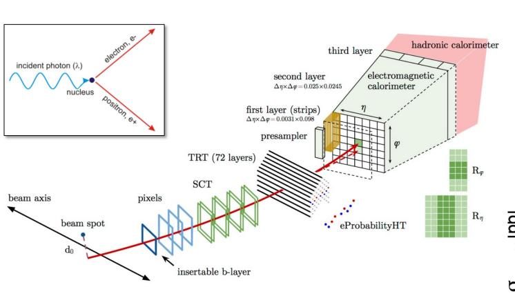
Photons (or converted to two electrons) without (with) track in internal detector, deposit energy in an electromagnetic calorimeter and then form a shower.
