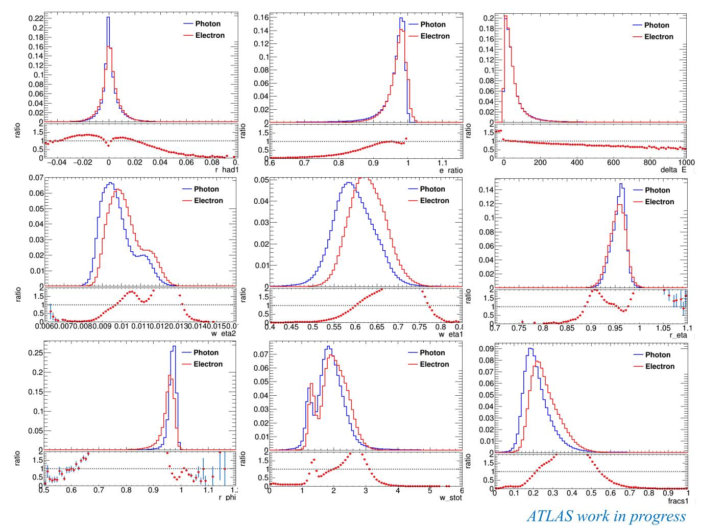
The identification of photons in ATLAS is achieved using a cut-based algorithm that applies a group discriminating variables.
