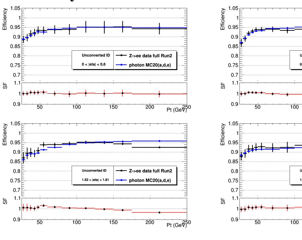
Scale factors are defined as ID efficiency of data divided by ID efficiency of MC. In most eta and P<sub>T</sub> bins, scale factors are close to 1.
