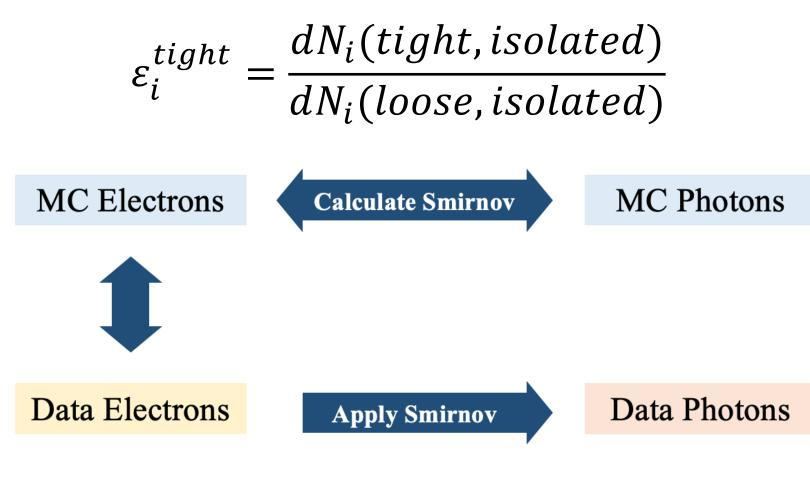
Based on the similarity of electron and photon shower shapes distortion in calorimeter, transform the electron shower shapes into photon-like by Smirnov transformation. Then measure the photon ID efficiency by those photon-like sample.
