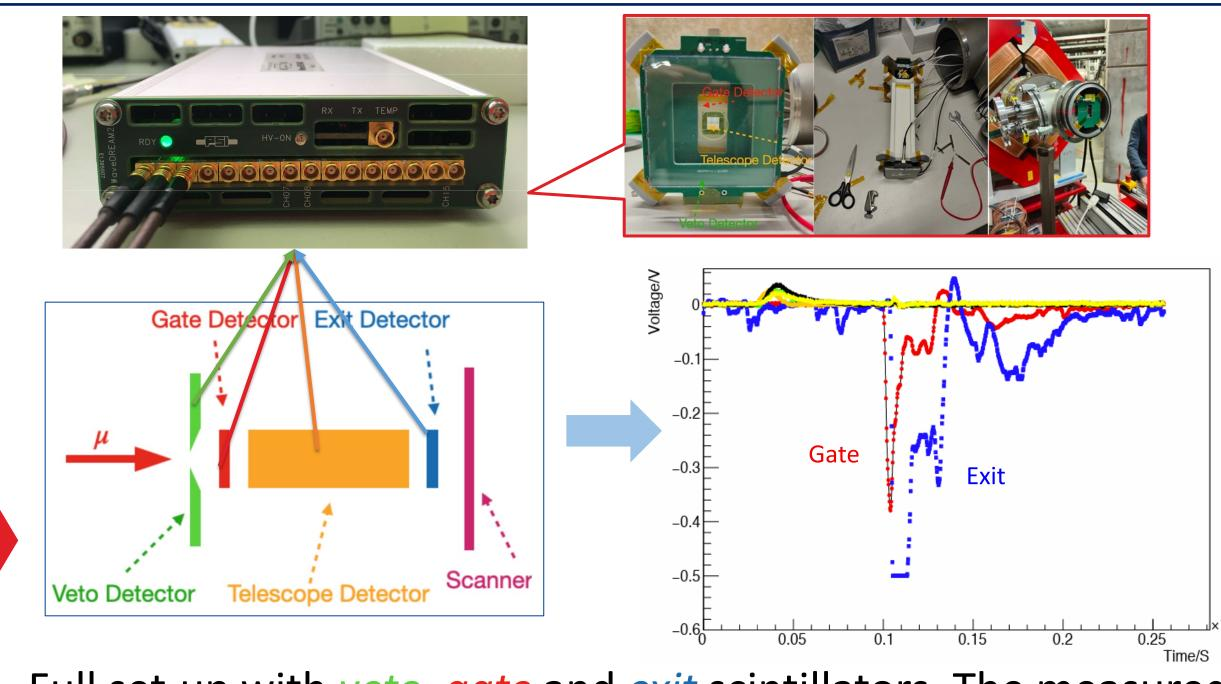
Full set-up with veto, gate and exit scintillators. The measured typical pulse signals of each sub-detectors allowed several trigger modes for better event characterization.
