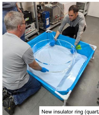
New insulator ring (quartz)
