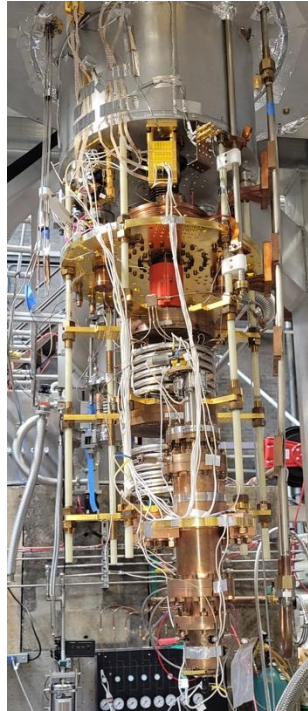
Dilution refrigerator + film burner (75 mW at 250 mK)
