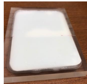
1/3 rd scale prototype side wall with embedded LiOH absorber and optical reflector
