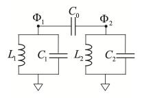
Use an additional capacitor to couple two LC circuits:
