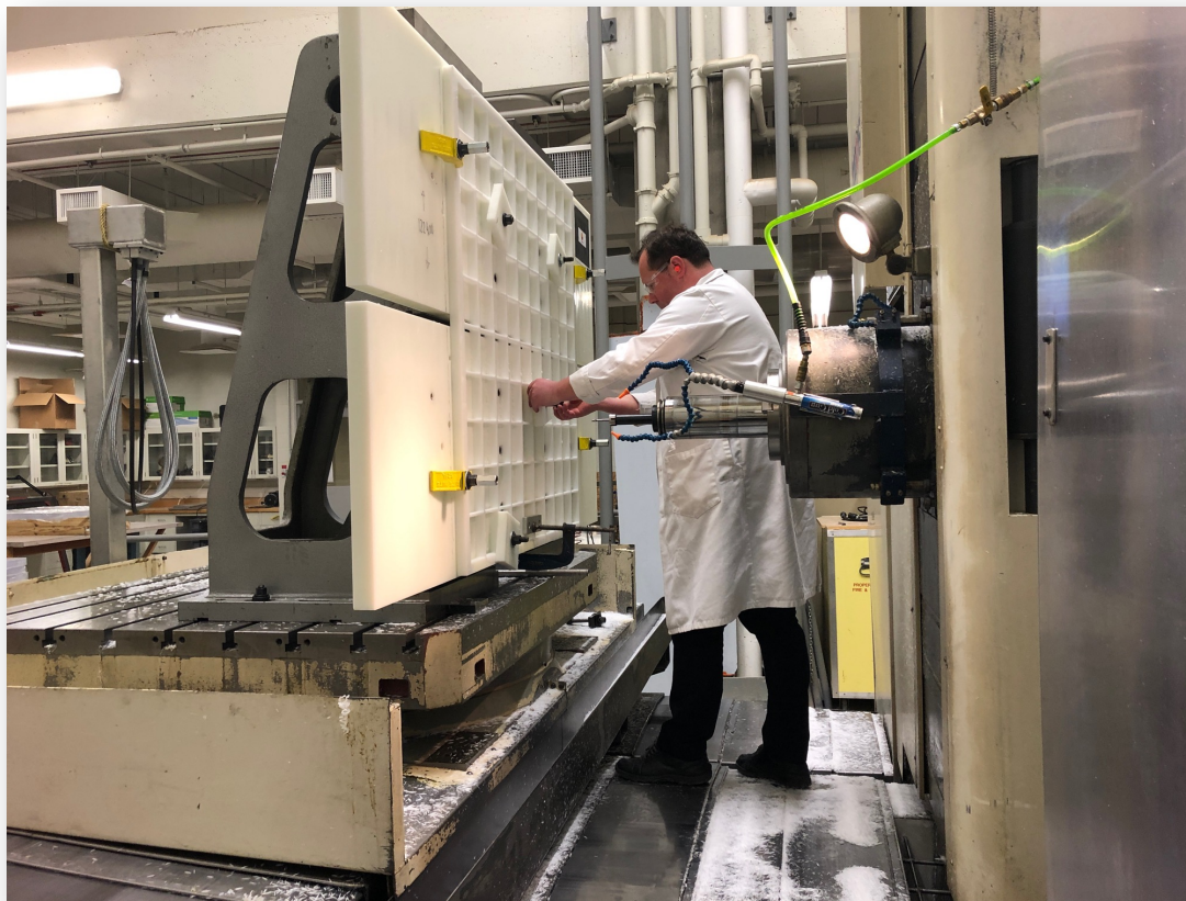
MAPP-mQP support structure being machined at the University of Alberta
