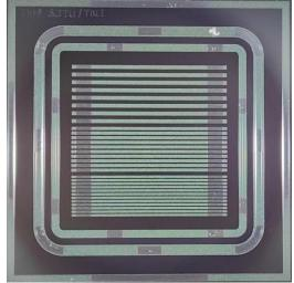
AC-LGAD silicon strip sensor 1x1 mm<sup>2</sup> designed, in collaboration with IHEP
